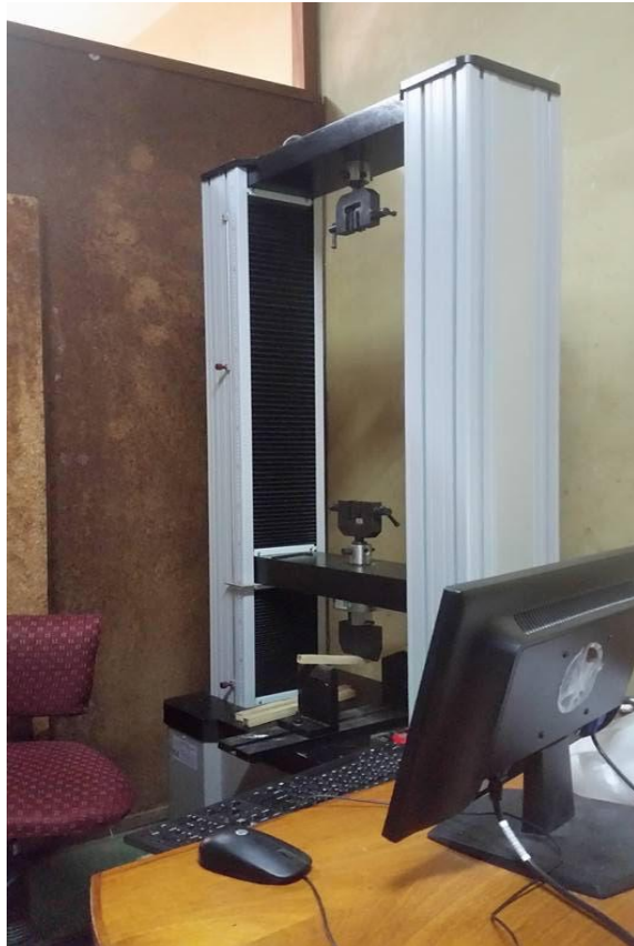
Fig. 2. Computer control electronic universal testing machine
