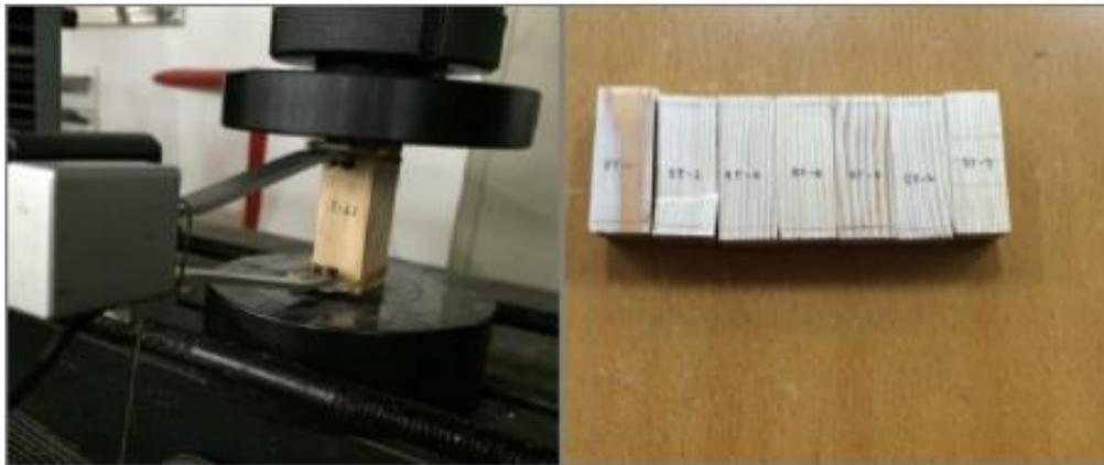
**Fig. 4.** Test for the modulus of elasticity in compression parallel to grain of wood
