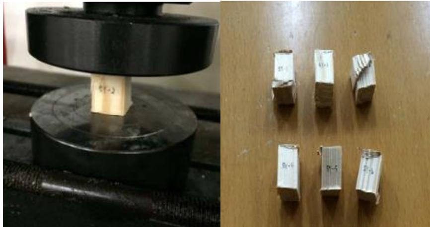
**Fig. 3.** Compressive strength test of timber
