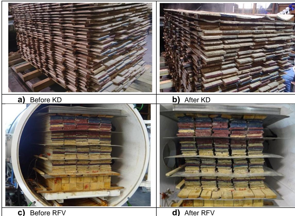
Fig. 2. Wood specimens during the drying process
