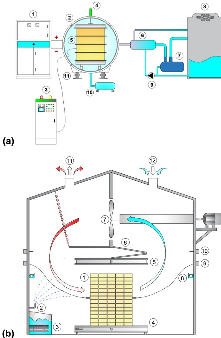
**Fig. 1.** (a) RFV dryer: 1) RF generator, 2) autoclave, 3) PLC and fiber optic sensor, 4) hydraulic press, 5) wood, 6) cooling tank, 7) vacuum pump, 8) cooling tower, 9) water pump, 10) condensate tank, 11) load cells. (b) KD dryer: 1) wood, 2) sprinkler, 3) evaporation tub, 4) balance, 5) counterbalance, 6) baffle, 7) fan, 8) wet-bulb temperature sensor, 9) wood temperature sensor, 10) dry-bulb temperature sensor, 11) and 12) are vents.
