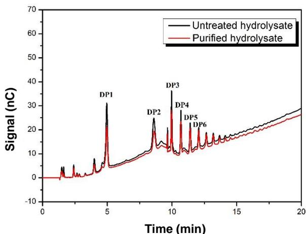
**Fig. 5.** Distribution of the degree of sugar polymerization in untreated hydrolysate and purified hydrolysate
