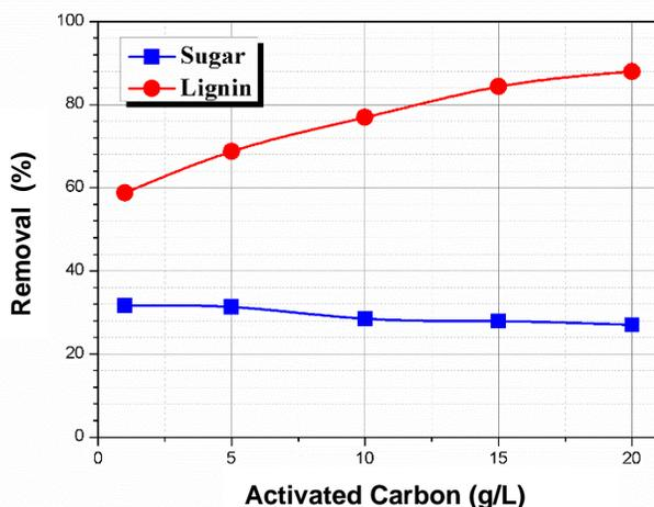
**Fig. 3.** The removal percentages of lignin and sugars with different levels of activated carbon during adsorption treatment
