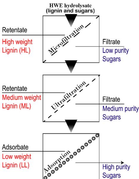
**Fig. 1.** The schematic flow diagram that describes the separation of sugar and lignin from HWE hydrolysate by the combined process of microfiltration, ultrafiltration, and activated carbon adsorption
