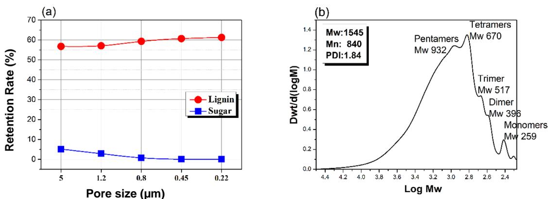
**Fig. 2.** Microfiltration of the HWE hydrolysate using membranes with different pore sizes: (a) performance of microfiltration in terms of lignin retention and sugars retention; (b) molecular weight distribution of HL obtained from microfiltration
