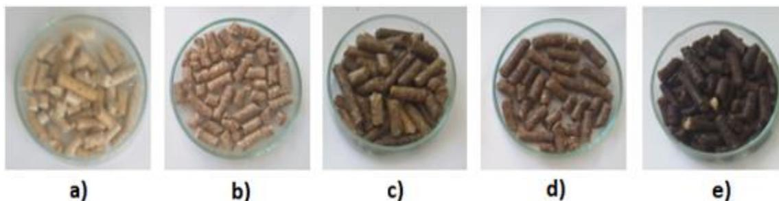
**Fig. 1.** Pellet samples: a) Spruce wood; b) Corn husks; c) Lawn clippings; d) Pine needles; and e) Linden leaves
