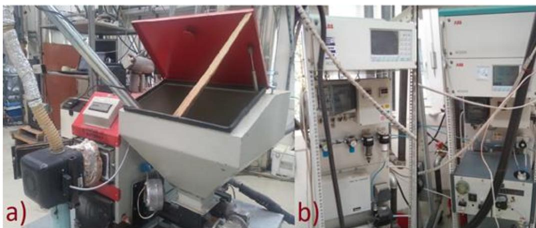
**Fig. 2.** The experimental combustion equipment: a) Boiler with burner; and b) Emission measuring devices
