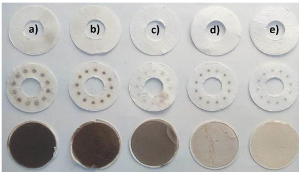
Fig. 11. The PM sedimentation filters: a) Pine needles; b) Linden leaves; c) Lawn clippings; d) Corn husk; and e) Spruce wood
