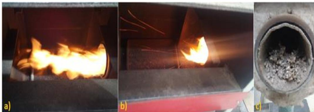
**Fig. 8.** The combustion process: a) Standardized burner operation; b) Burner clogging; and c) Clogged rotary burner after the combustion of alternative biomass samples
