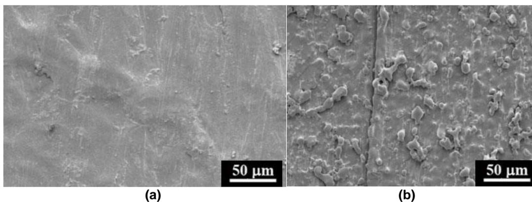
Fig. 2. The microstructure of different rice husk detected by SEM: a: US and b: SE-2.5
