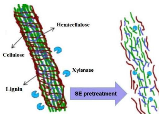
**Fig. 1.** The schematic of SE-pretreated cell wall of rice husk
