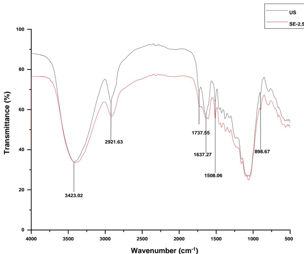
Fig. 3. FTIR spectroscopy of SE-pretreated rice husk
