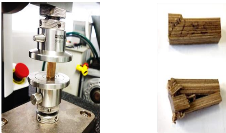
Fig. 5. Compression discs and failures in the compression specimens
