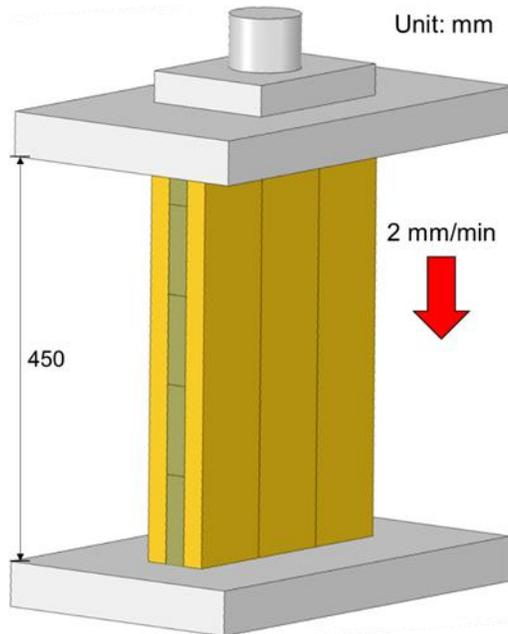
Fig. 3. Schematic diagram of compressive strength test and 200t UTM
