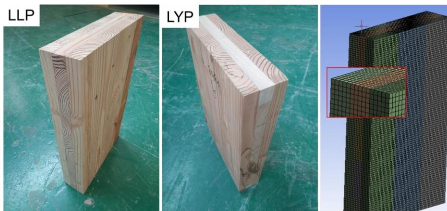
Fig. 4. CLT photograph and FEM-model structure
