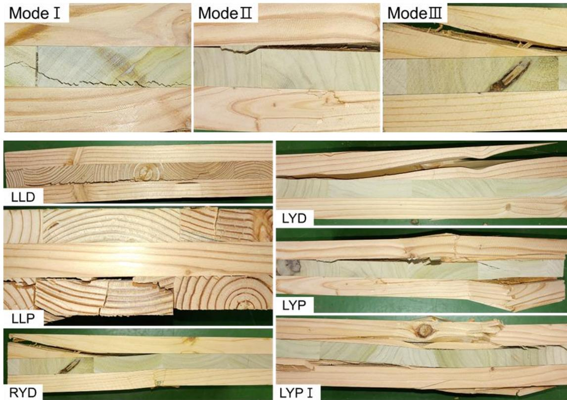
Fig. 6. Failure modes of CLT specimens
