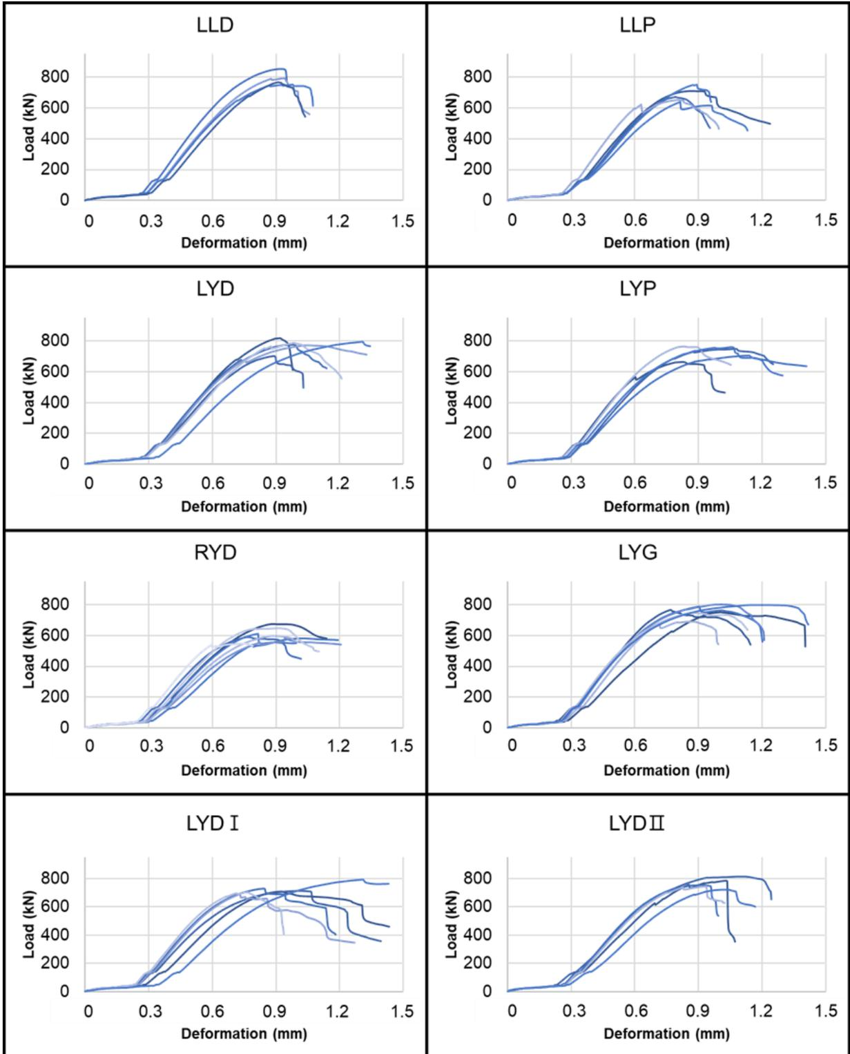
Fig. 5. Load-deformation response for CLT specimens
