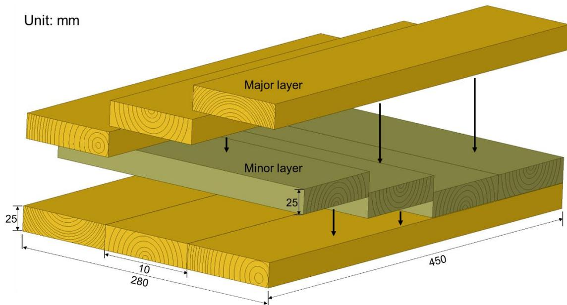
Fig. 2. Schematic diagram of cross-laminated timber
