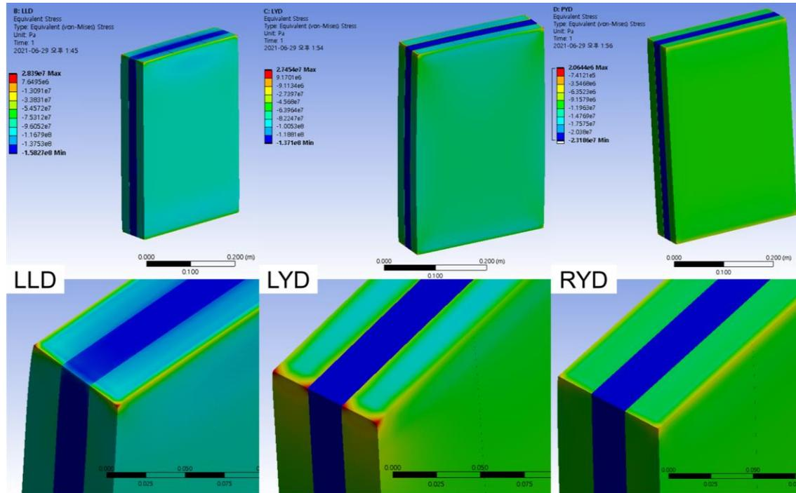
**Fig. 7.** Stress distribution of CLT specimens under compressive load calculated by FEM analysis
