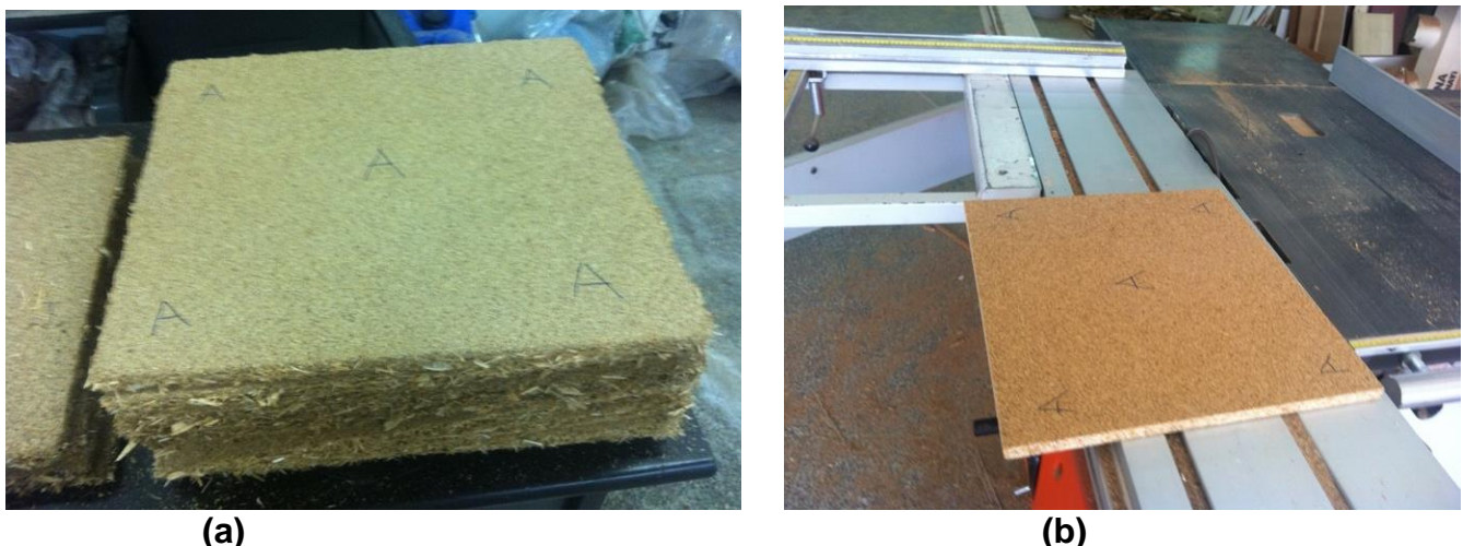
Fig. 1. (a) Composites produced from HTT WS and UT WS and wood; (b) trimmed composites
