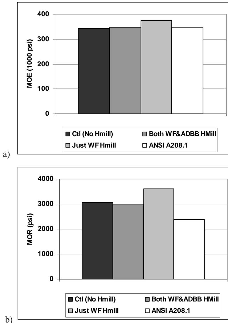
**Figure 1.** Effects of pre-process hammermilling of fiber on a) Modulus of Elasticity (MOE) and b) bending strength (MOR) of 50/50% hybrid wood-ADBF dry-formed fiberboard compared to commercial H-1 grade particleboard requirements.
