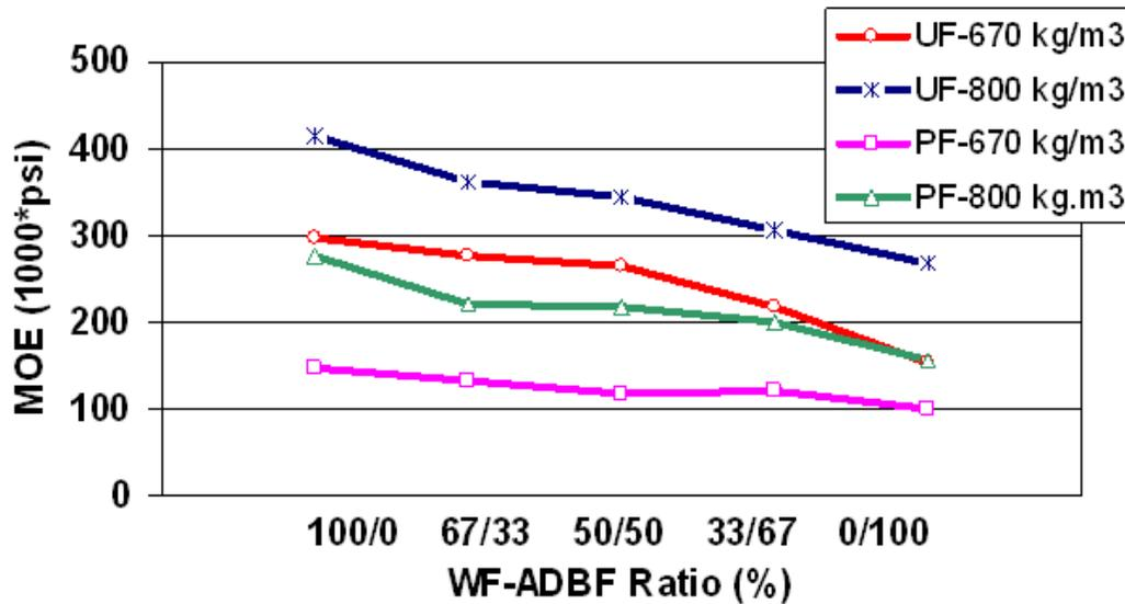
Figure 2. Effects of various WF and ADBF fiber mixtures and fiberboard density on Modulus of Elasticity (MOE)
