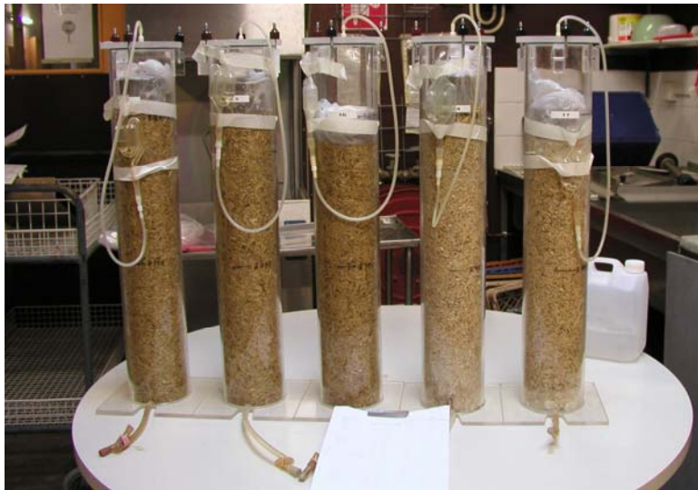
Fig. 1. Storage of chemically pretreated wheat straw in Plexiglass® acrylic silos. Sealing with Plexiglass® plate, lead weight, and water seal.
