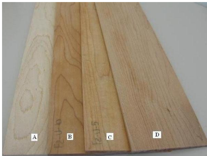
Fig. 1. EB cure impregnated sugar maple samples: (A) Control; (B) 10 min vacuum; (C) 5 min vacuum; and (D) 15 min vacuum/15 min pressure
