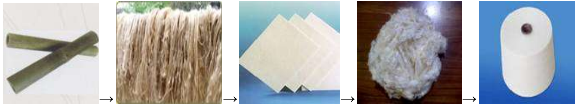
From left to right: (1) raw bamboo is gathered, (2) bamboo is crushed and processed into thick pulp (raw chemical bamboo fibre) (Pure Fiber 2008), (3) bamboo is further processed into fine pulp sheets, (4) bamboo pulp is manufactured into fibre through wet spinning process, (5) bamboo fibres are spun into yarn
