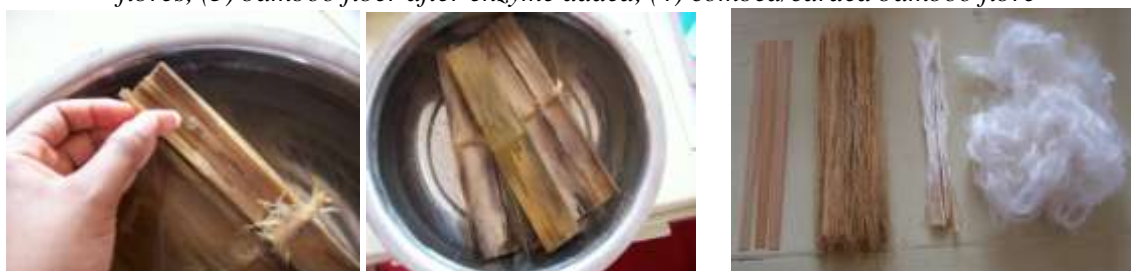
Figure 3.2b: Mechanical Bamboo Fibre Manufacturing (Lin 2008) Left and centre photographs: cut bamboo culm boiled to remove inner fibres; Right photograph, from left to right: (1) post-boiled inner bamboo strips, (2) crushed bamboo fibres, (3) bamboo fiber after enzyme added, (4) combed/carded bamboo fibre
